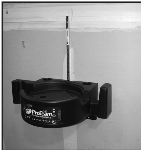
The proper height of the ProTeam Vac Station is determined by the user of the vacuum. The vacuum user should be able to back up to the Vac Station and without bending his or her knees or rising on the balls of his or her feet, slip the vacuum on or off of the Vac Station easily.
